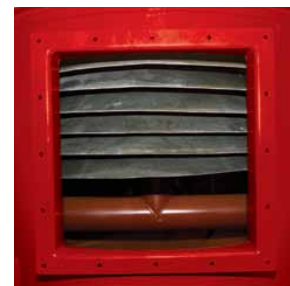
Innovative separating baffles are made of corrugated fiberglass infused with epoxy for long life. An access plate allows easy maintenance of the baffle and float assemblies.
