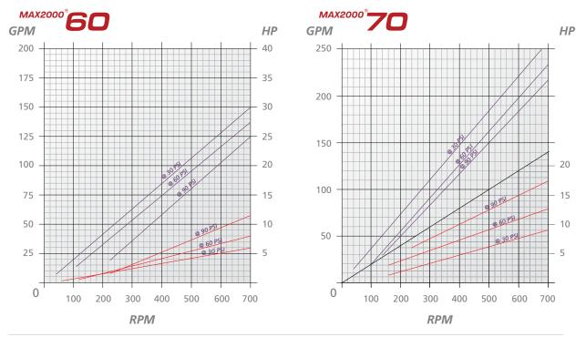
The information contained herein is based on a theoretical calculation of rotor/stator geometry. Based on water at 70°F.
