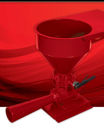
The MAX2000<sup>®</sup> 6" Mud Hopper by PSI is a rugged low-pressure, high-volume unit that makes it easy to accurately mix solids additives into drilling fluid. Fed by a 40 to 60 PSI mud system centrifugal pump at a volume of 1100 to 1400 gallons per minute.
