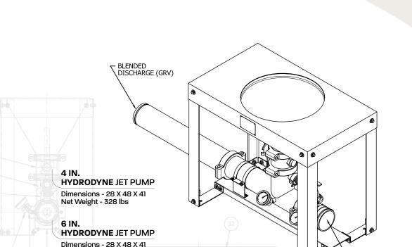
In short, our all-weather, high shear hoppers mix your materials quickly with the liquid/additive of your choice using low pressure loss, thus minimizing fish eyes and eliminating the need for extra equipment. They reduce the amount of waste needing disposal and minimize the environmental impact of that waste.
