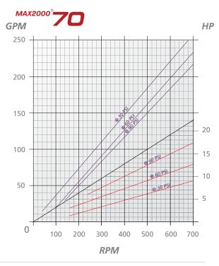
The information contained herein is based on a theoretical calculation of rotor/stator geometry. Based on water at 70°F.
