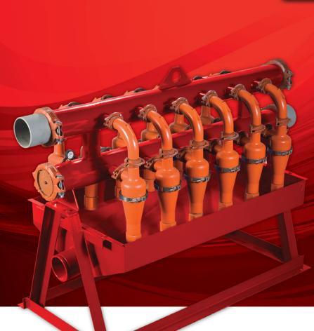
PSI hydrocyclone units deliver efficient, economical and dependable services for separation of solid-phase particles in the drilling fluid. Built on a easily moved skid, the units include mud trough, manifold, polyurethane hydrocyclones, pressure gauge and all necessary connections.
