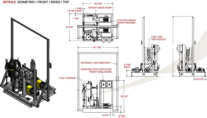
In short, the MAX2000<sup>®</sup> Fuel Filtration System offers a highly efficient and reliable way of filtering fuel until it's practically free of contaminants. The back-up pump ensures no downtime — thereby reducing income loss, and the explosion-proof starters and motors maximize personnel protection in challenging settings.
